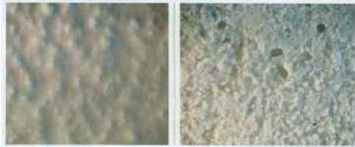
Left: 14X magnification of plaster coupon in pool with 0 ppm cyanuric acid
